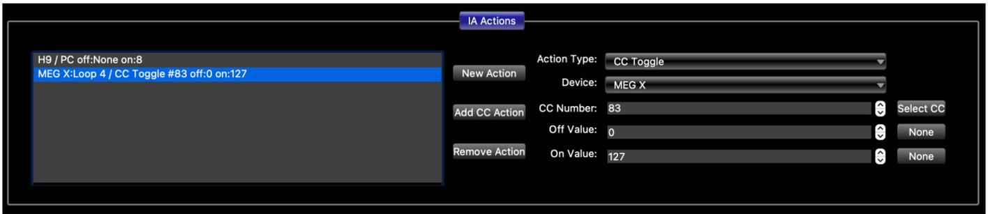
To control a Mastermind PBC loop: In each button that controls your effect, add a second action that controls the loop containing your effect. Press **New Action**, then set **Action Type** to **Audio**. Next, set **Subtype** to **Loop** and set your loop number. Make sure **Off Value** is set to OFF and **On Value** is set to ON.
