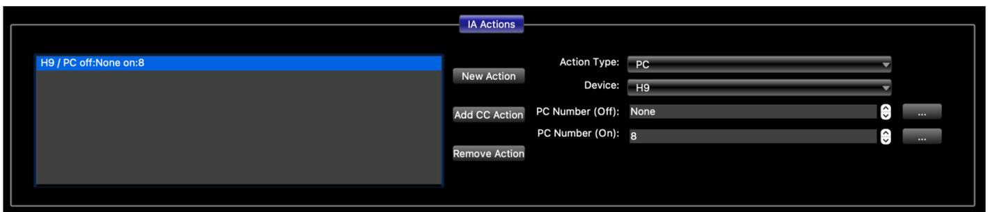
Repeat this for each button you wish to set up to send PCs to your device. Make sure that each of these buttons is assigned the same group number. This will insure that only one button in the group can be on at any time.
