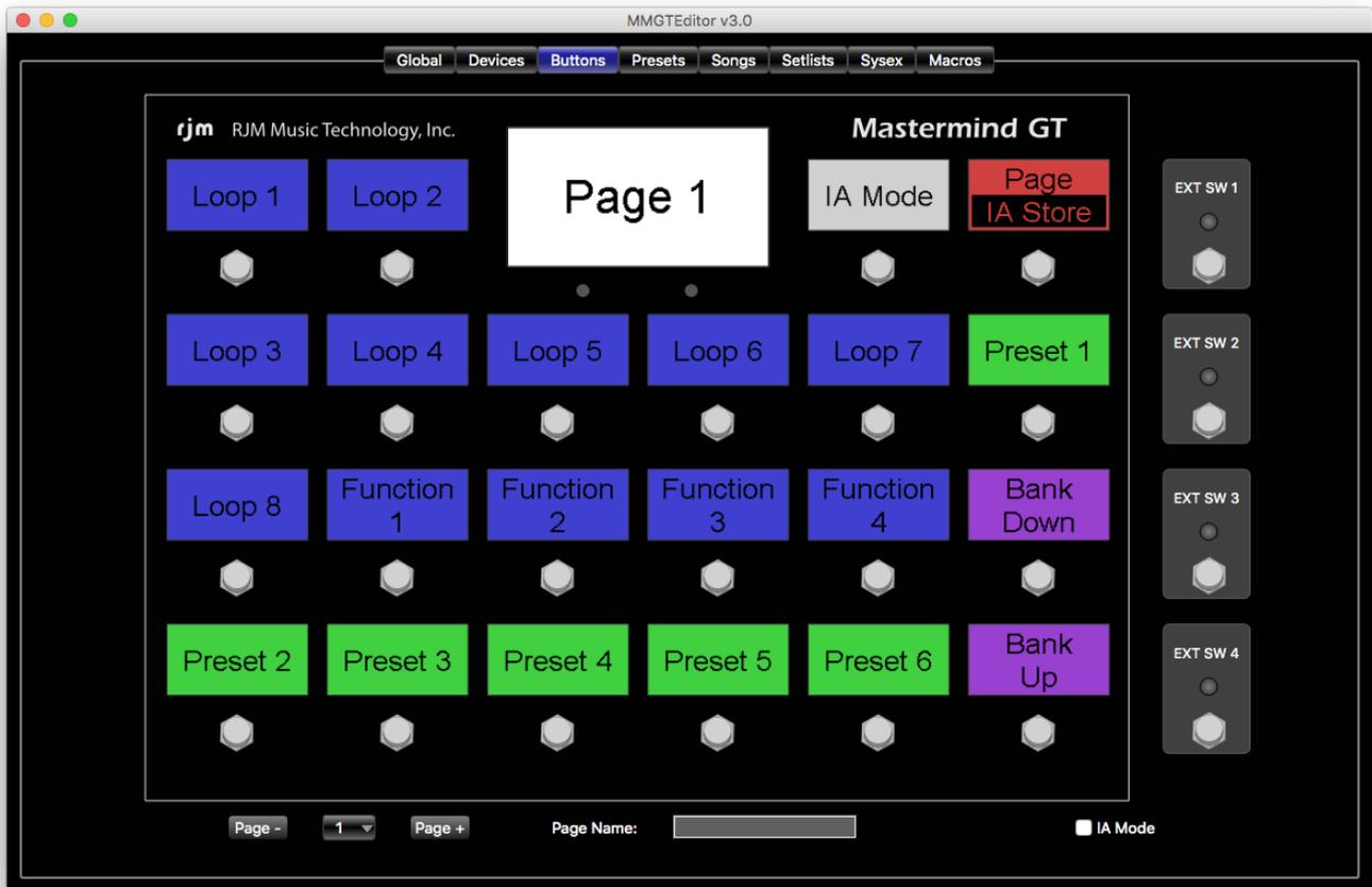
One of the most important features of the Mastermind GT, LT and PBC is the ability to redefine buttons. Any button can be changed to perform any function, and you can have multiple pages of buttons with different button configurations.
