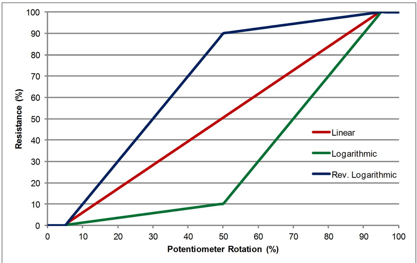
The red line indicates a linear taper - it's a straight line all the way across. The green line is a logarithmic taper. Note that it has a "knee" where the line breaks and heads upward at a steeper slope. This is where the **Taper X** and **Taper Y** values come in.
